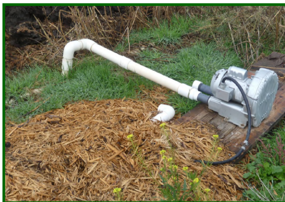
An air pump that pulls or pushes air into a municipal treated waste and compost mixture to heat the compost to 120 degrees to kill weed seed .
