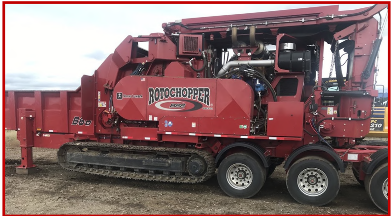
Traveling shredder that grinds yard waste into compost
